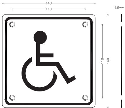
DISABLED TOILET DOOR SIGN - MATERIAL: STAINLESS STEEL EN 1.4301 (TYPE 304) SIZE: 140X140X1.5 MM - SUPPLIED WITH WOOD & STEEL SCREWS
