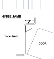
Note: Installing in different layout around the door jamb (head, hinge jamb, & strike jamb) is applicable as long as the door would be able to operate properly.
