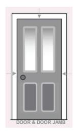
Seal gap between door and door jamb. Apply to Top part and both sides of the door jamb. Installation Guidelines for **DS88** Adhesive Gasketing
